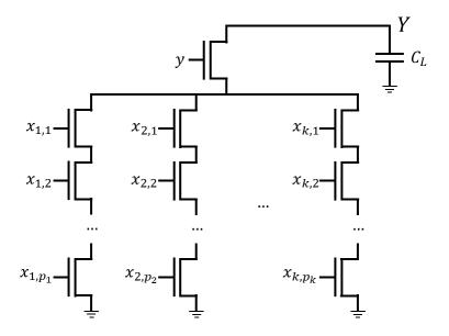
(5) [**Design, 20 points**] The following (in the next page) shows an NFET network of Y in Problem 4. Size the transistors so that the fall delay is less than or equal to  $R_nC_L$  where  $R_n$  is the resistance of a 1X NFET. Minimize the total width. Find the total width.
