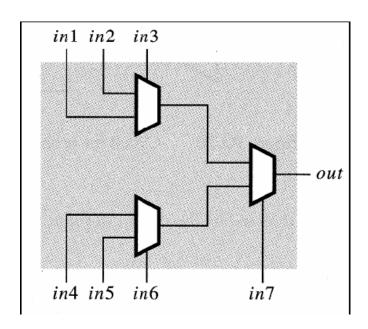
Show how the logic cell can be used to realize  $f = X_1 \cdot X_2 + X_3$ Show how the logic cell can be used to realize  $f = X_1 \cdot X_3 + X_2 \cdot X_3$
