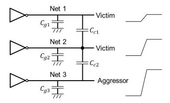
Net 3 is the only aggressor and Net 2 and Net 1 are victims. Although Net 1 is not directly connected to Net 3, Net 1 is affected by the potential change of Net 2 when Net 3 switches. The above figure can be simplified as follows:
