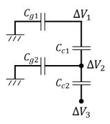
1 – 13 points) Derive  $\Delta V_2$  and  $\Delta V_1$  as a function of  $\Delta V_3$ ,  $C_{g1}$ ,  $C_{g2}$ ,  $C_{c1}$ , and  $C_{c2}$ .
