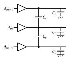
1-10 points) Compute effective capacitance for the net in the middle  $(d_m)$  for the following transition patterns:
