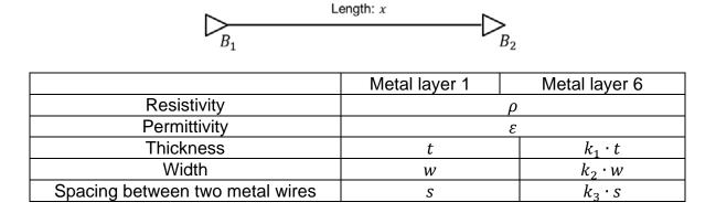
The wire is sufficiently long, so you can ignore the input capacitance of B2. You can also assume that the output resistance of B1 is very small (almost zero ohm).
