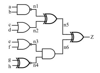
1) Find all test vectors that can detect a s-a-0 fault at input f. (You can use X for don't-cares).
