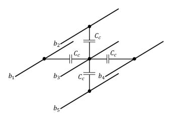
Due to the coupling between  $b_3$  and  $b_k$ , the worst-case effective coupling capacitance that  $b_3$  experiences will be  $8 \cdot C_c$ . List all transition patterns that make  $b_3$  experience  $8 \cdot C_c$  and  $7 \cdot C_c$ .
