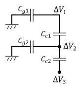
1 – 12 points) Derive  $\Delta V_2$  and  $\Delta V_1$  as a function of  $\Delta V_3$ ,  $C_{g1}$ ,  $C_{g2}$ ,  $C_{c1}$ , and  $C_{c2}$ .
