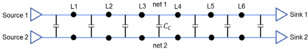
Two nets (net 1 and net 2) are coupled as shown above and you are supposed to insert a repeater (inverter or buffer) into each of the designated locations (L1 ~ L6). For instance, the following figure shows a repeater insertion solution (its delay and area are  $12d$  and  $20S$ , respectively):
