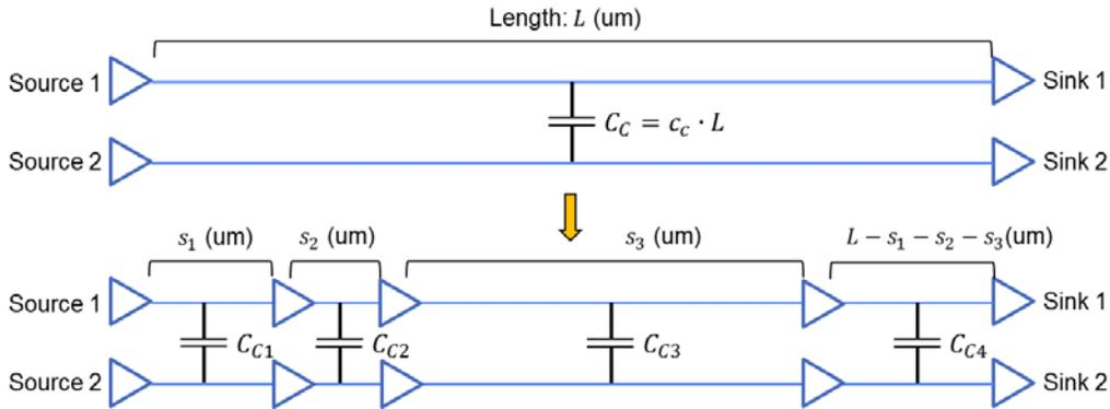
Two nets are routed as shown above. The coupling capacitance between them is  $C_c$ . You are supposed to insert buffers into the nets identically as shown above. All the drivers, sinks, and buffers are of the same type. The following list shows all the parameters and variables you should use:
