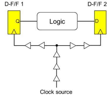
There are five buffers between the clock source and the clock pin of D-FF1 (and D-FF2) as shown in the figure. Ideally, the following inequalities should be satisfied:
