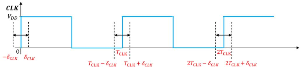
Derive a new setup time and a new hold time constraints (inequalities) that should be satisfied under the variations.
