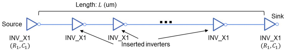
A buffer is composed of two inverters, so it consumes more power than an inverter. Thus, we can insert inverters instead of buffers to optimize a net while minimizing power consumption. However, only an even number of inverters can be inserted (if the inverter count is odd, there will be signal inversion).
