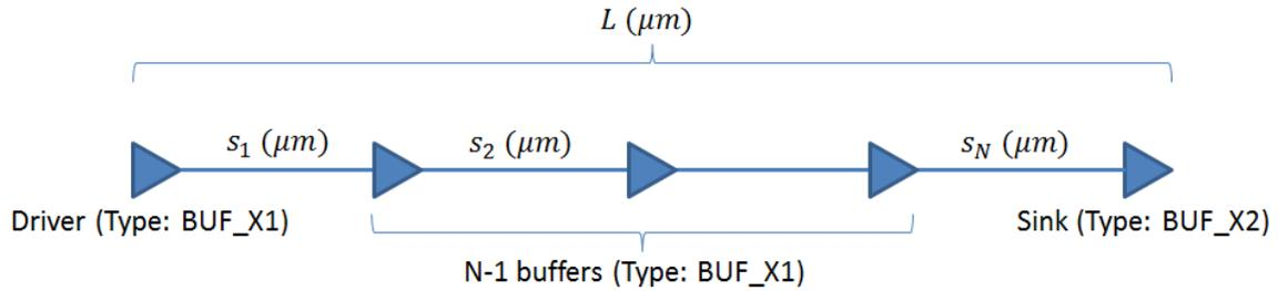
A source (type: BUF\_X1) drives a sink (type: BUF\_X2) through a net and you are supposed to optimally insert  $N-1$  buffers (type: BUF\_X1) between them. Find the number of buffers to insert (i.e., find  $N$ ) and the optimal locations of the buffers (i.e., find  $s_1, s_2, \dots, s_N$ ) minimizing the total delay.
