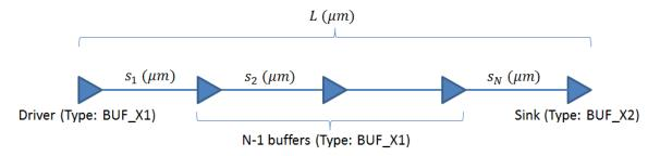
A source (type: BUF\_X1) drives a sink (type: BUF\_X2) through a net and you are supposed to <u>optimally</u> insert N-1 buffers (type: BUF\_X1) between them. <u>Find the number of buffers to insert (i.e., find N) and the optimal locations of the buffers (i.e., find  $s_1, s_2, ..., s_N$ ) minimizing the total delay.</u>
