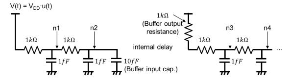
In this case (inserting a buffer into n2), the delay at  $V_{L1}$  is  $[1k*11f+1k*12f+\cdots+1k*29f+1k*59f+1k*60f+\cdots+1k*77f+1k*77f]+[20ps]+[1k*11f+1k*12f]=(1749+20+23)ps=1792ps$ , so is the delay at  $V_{L2}$ . As you see, the delay is reduced from 1829ps to 1792ps.
