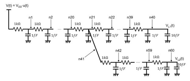
Currently, the delay at  $V_{L1}$  is  $1k * 11f + 1k * 12f + \cdots + 1k * 29f + 1k * 59f + 1k * 60f + \cdots + 1k * 79f = 1829ps$ , so is the delay at  $V_{L2}$ .
