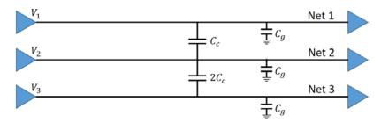
The figure shows three parallel nets. The coupling capacitance between Net 1 and Net 2 is  $C_C$ . The coupling capacitance between Net 2 and Net 3 is  $2C_C$ . The following shows a three-bit binary encoding technique for four decimal numbers (0, 1, 2, 3).
