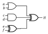
(1) Find all input vectors that can detect a s-a-0 fault at input a. (10 points)
