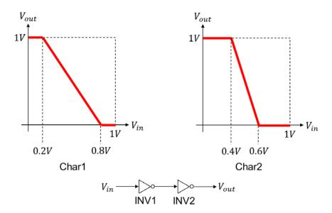
The gate-level schematic shows a buffer composed of two inverters.
