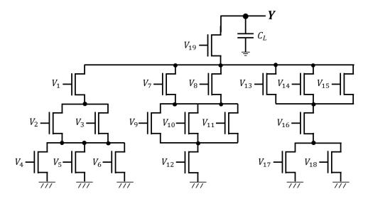
All the transistors in the figure shown above have the same width W. Ignore parasitic RC. All the inputs are 0V at time 0. At time t, some of the input voltages switch from 0 to  $V_{DD}$ . Which one of the following has the smallest falling delay?
