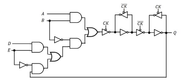
This logic gate is a flip-flop (D is a data input, CK is a clock input, and A, B, E are some additional inputs.) Describe the functionality of the flip-flop in as much detail as possible (e.g., whether it is positive-edge-triggered, negative-edge-triggered, or dual-edge, and what A does, etc.).
