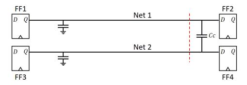
The following figure shows two waveforms when a crosstalk occurs between Net 1 (aggressor) and Net 2 (victim). If the potential of Net 2 is higher than  $0.1V_{DD}$ , signal inversion could happen in Net 2.
