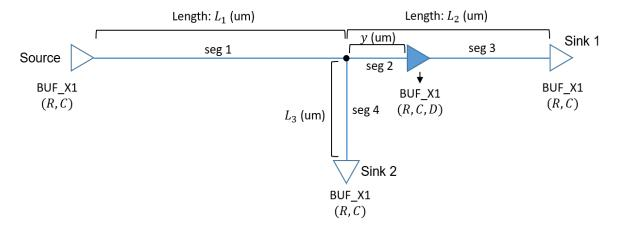
(4) Replace each segment (seg 1, 2, 3, 4) by a PI model. Then, express the delay from the source to Sink 1 using the Elmore delay model. (10 points)
