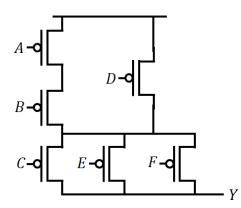
Size the transistors in the NFET network (show the size of each TR below). Timing constraint:  $\tau_r \leq 0.25 R_n C_L$  ( $\tau_r$  is the rise delay). Try to minimize the total transistor width.
