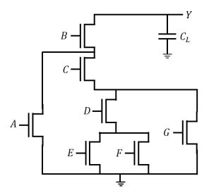
Size the transistors in the NFET network (show the size of each TR below). Timing constraint:  $\tau_f \leq R_n C_L$  ( $\tau_f$  is the fall delay). Try to minimize the total transistor width.
