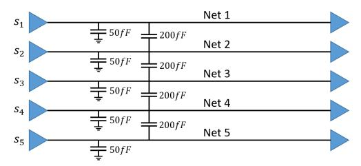
This figure shows a bus composed of five nets. The following shows the data we are going to transfer through the bus:
