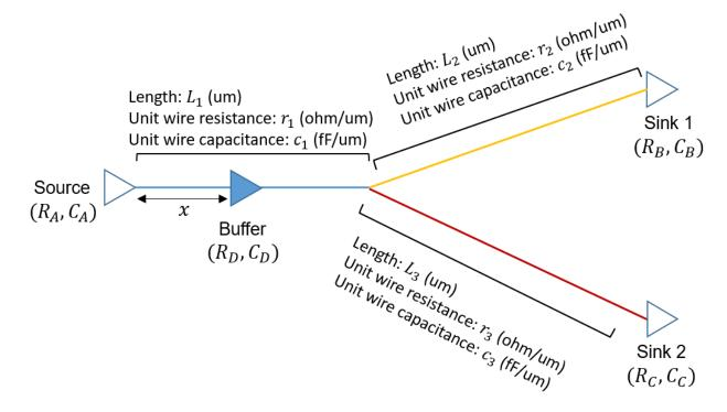
Notice that (R, C) is the (output resistance, input capacitance) of the corresponding cell. x is the optimal location of the buffer  $(0 < x < L_1)$ . We ignore the internal delay of the buffer. Use the PI model for each wire segment for delay estimation. We want to minimize the delay from the source to Sink 1 in this problem.
