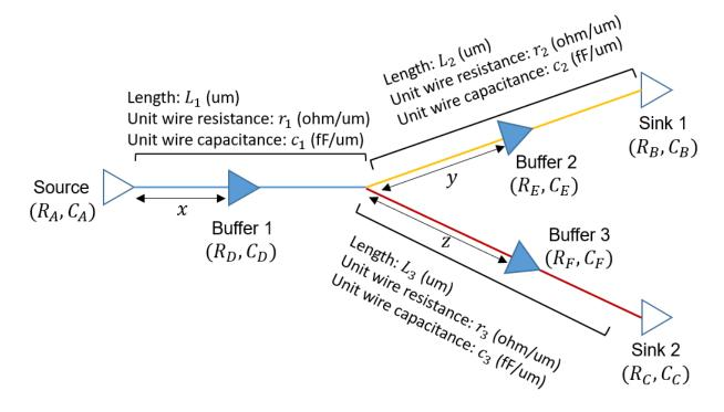
Notice that (R,C) is the (output resistance, input capacitance) of the corresponding cell. x,y,z are the optimal locations of Buffer 1, 2, 3, respectively  $(0 < x < L_1, 0 < y < L_2, 0 < z < L_3)$ . We ignore the internal delays of the buffers. We want to minimize both the delay from the source to Sink 1 and the delay from the source to Sink 2 in this problem.
