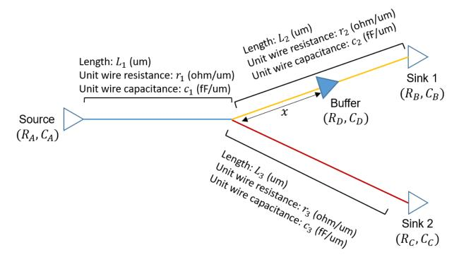
Notice that (R,C) is the (output resistance, input capacitance) of the corresponding cell. x is the optimal location of the buffer  $(0 < x < L_2)$ . We ignore the internal delay of the buffer. Use the PI model for each wire segment for delay estimation. We want to minimize the delay from the source to Sink 1 in this problem.
