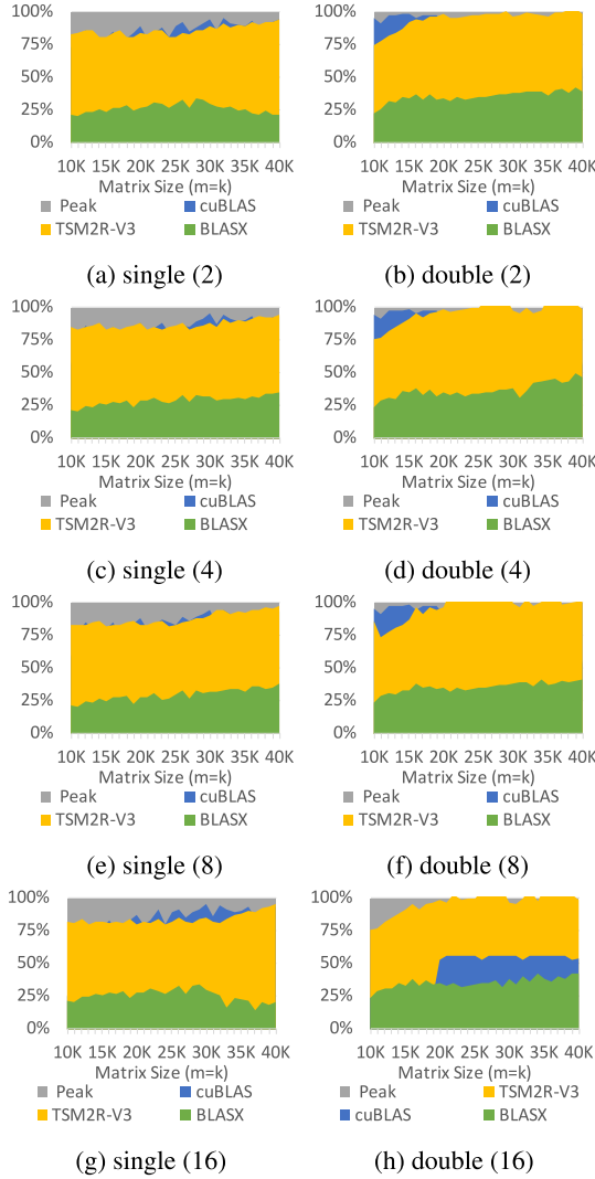
Fig. 11. Memory bandwidth utilization with single and double precision on V100 ( n = 2, 4, 8, 16 ).
