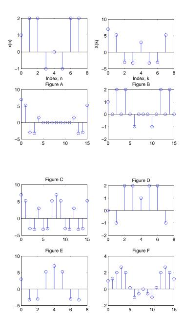
2. (15 points) Which of the following is the impulse response of a causal, linear-phase FIR digital filter? Proper justification must be provided to receive credit.
