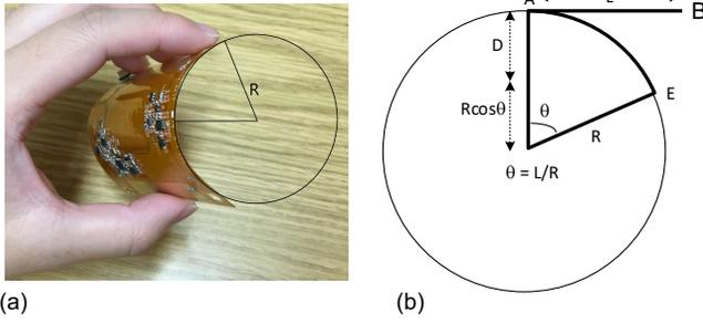
Fig. 3. Determining required displacement,  $D$ , from the given bending specifications as radius of curvature,  $R$ , and the cantilever length,  $L$ .
