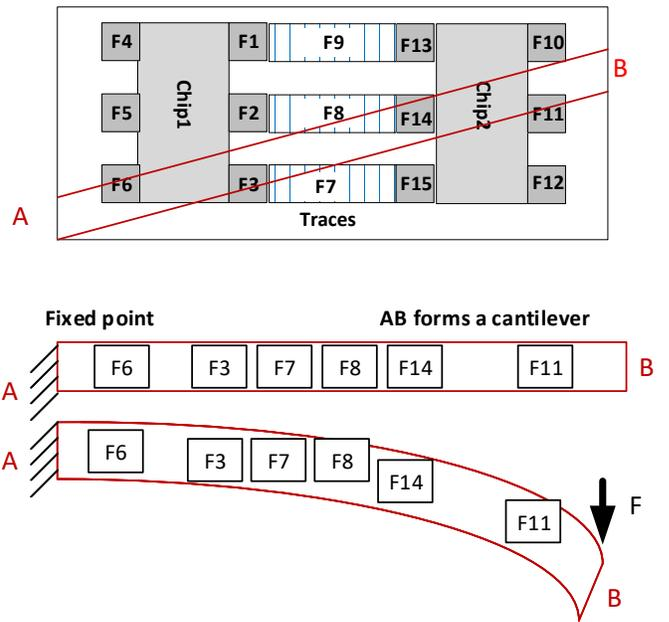
Fig. 1. An illustrative example of an FHE board with rigid components, solder joints, and traces generating potential parametric and catastrophic faults along the chosen mechanical stress pattern AB.
