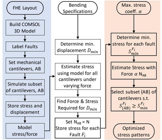
Fig. 2. Flow of the proposed mechanical stress optimization methodology
