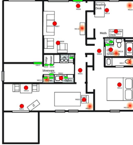
●: Motion sensor    ■: Area sensor    ■: Door sensor
