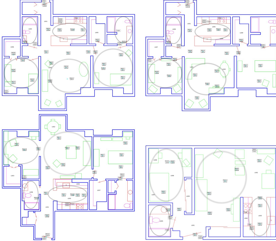
Fig. 2: Smart home testbed floorplans and sensor positions. Sensor labels starting with “M” are motion directors, “D” represents door sensors, “LS” represents light sensors, and “T” represents temperature sensors. From upper left, the testbed homes are labeled SH1, SH2, SH3, and SH4.
