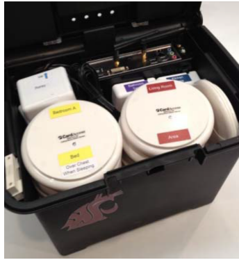
Fig. 1: CASAS SHiB. Downward-facing passive infrared motion detectors are installed inside the refrigerator, above each bed, each seating area, the kitchen sink, and the stove. Area motion detectors are placed in each large room. Magnetic door closure sensors are attached to external doors and selected cabinets. As sensors generate readings, the smart home adds timestamps and sensor identifiers to the readings and stores the data for later analysis.
