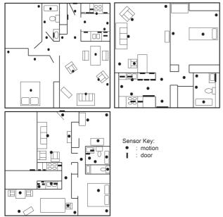
Figure 3. The sensor layouts (black circles) and doors (black rectangles) for the three apartments: B1 (top left), B2 (top right), and B3 (bottom)
