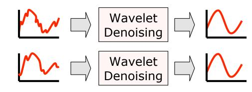
The time and scale resolution of the representation depends on the selection of a wavelet basis. By carefully choosing the basis function, the adverse effect of synchronization offset can be minimized.
