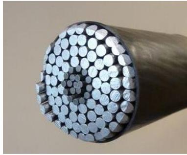
Fig. 2.2.4. Cross sectional view of a stranded aluminum conductor steel reinforced (ACSR) conductor (courtesy R. Aho, BPA). Note that the rubber coating is here only for the purpose of holding the sample together. Conductors in service will generally not have this coating.
