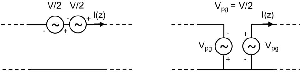
Fig. 7.9.1. a) circuit equivalent to a series source of voltage  $V$  b) equivalent phase to ground sources for the case that all cross sectional dimensions of the power line are small compared to a wavelength at the operating frequency.
