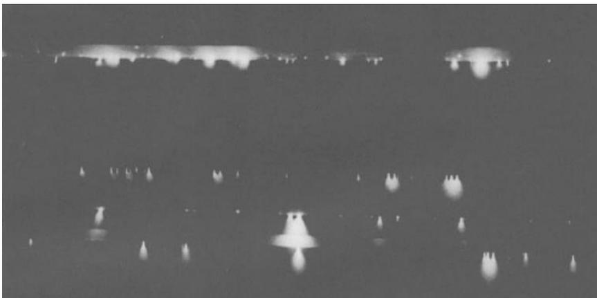
Fig. 1.6.3. The white spots are corona discharges randomly located along a conductor energized to high voltage
