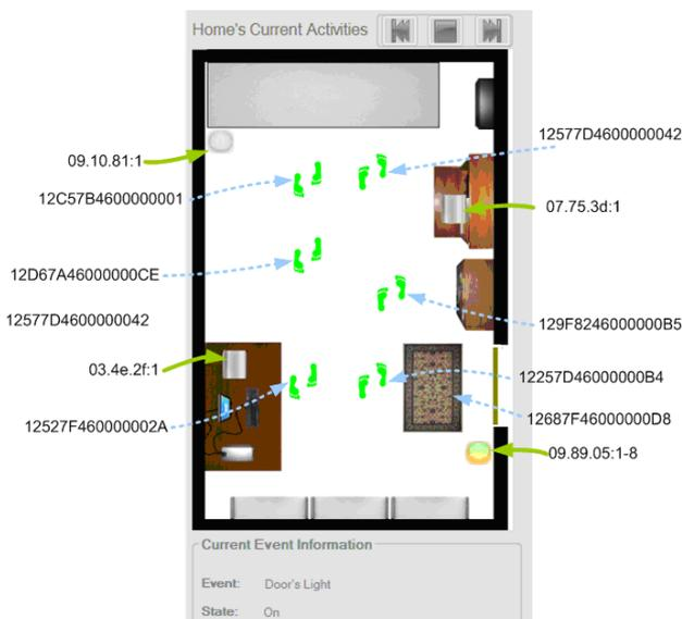
Figure 6: Sensor layout and floor-plan map.
