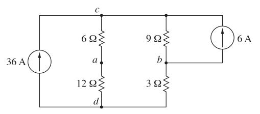
3. Use node-voltage analysis to find  $i_x$  in the circuit shown below.
