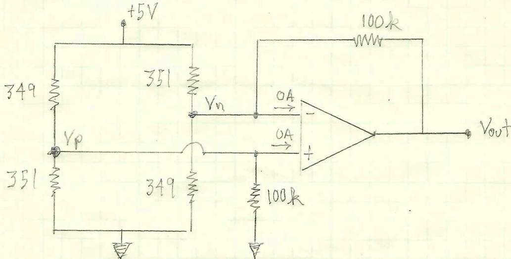
Can obtain voltage at  $V_p$  from voltage division. Note that the  $351\Omega$  resistor is in parallel with the  $100k\Omega$  at non-inverting terminal.
