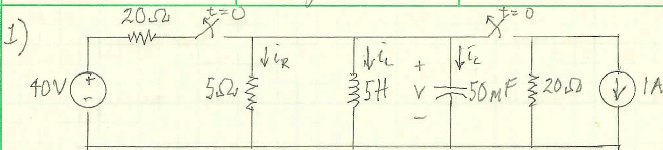
For  $t < 0$ , both switches are closed and the inductor appears as short circuit. Thus all current from voltage and current source flow through it, but in opposite directions.
