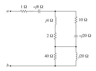
3. For the circuit below, the frequency  $\omega$  is 50,000 rad/s. The circuit is in sinusoidal steady state. What is the voltage  $v_1(t)$ ?
