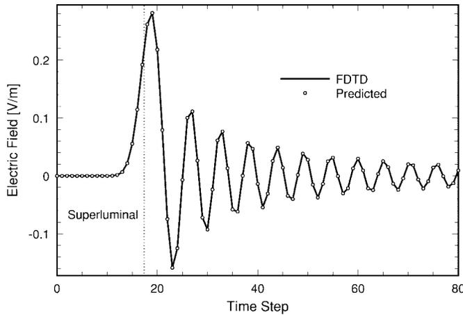
Fig. 2. Electric field ten cells away from a Kronecker delta source versus time. The boundary between super- and subluminal propagation is the dotted vertical line. The nonzero fields to the left of this line prove that the FDTD grid supports superluminal propagation.
