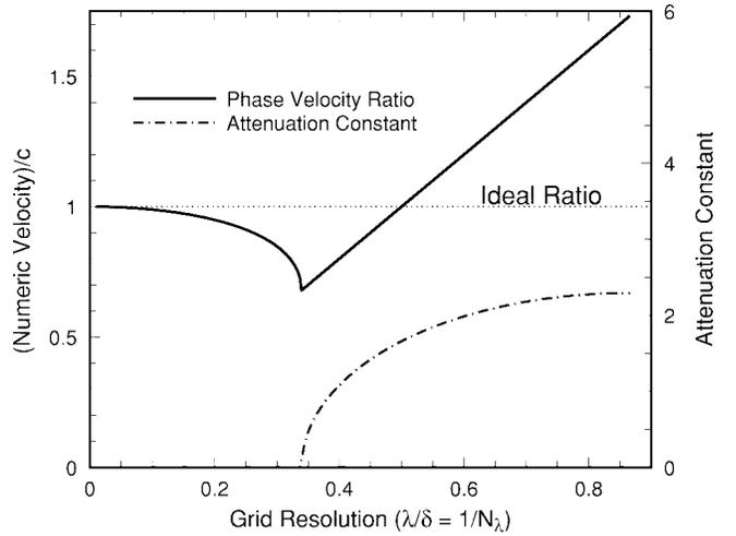
Fig. 1. Solid line is the ratio of the numeric phase velocity versus grid resolution ( $1/N_\lambda$ ). The Courant number is  $1/\sqrt{3}$  which gives a minimum  $N_\lambda$  of  $2/\sqrt{3} \approx 1.155$  or a maximum spatial step of  $0.866\lambda$ . The dash-dot line is the per-cell attenuation constant versus grid resolution.
