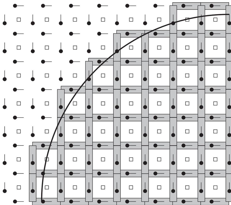
Figure 8.13:  $TE^z$  grid with a PEC object. The PEC is assumed to exist below and to the right of the curved boundary. The PEC is realized by setting to zero any electric field which has a neighboring  $H_z$  node within the PEC. The nodes that would be set to zero are surrounded by gray rectangles.
