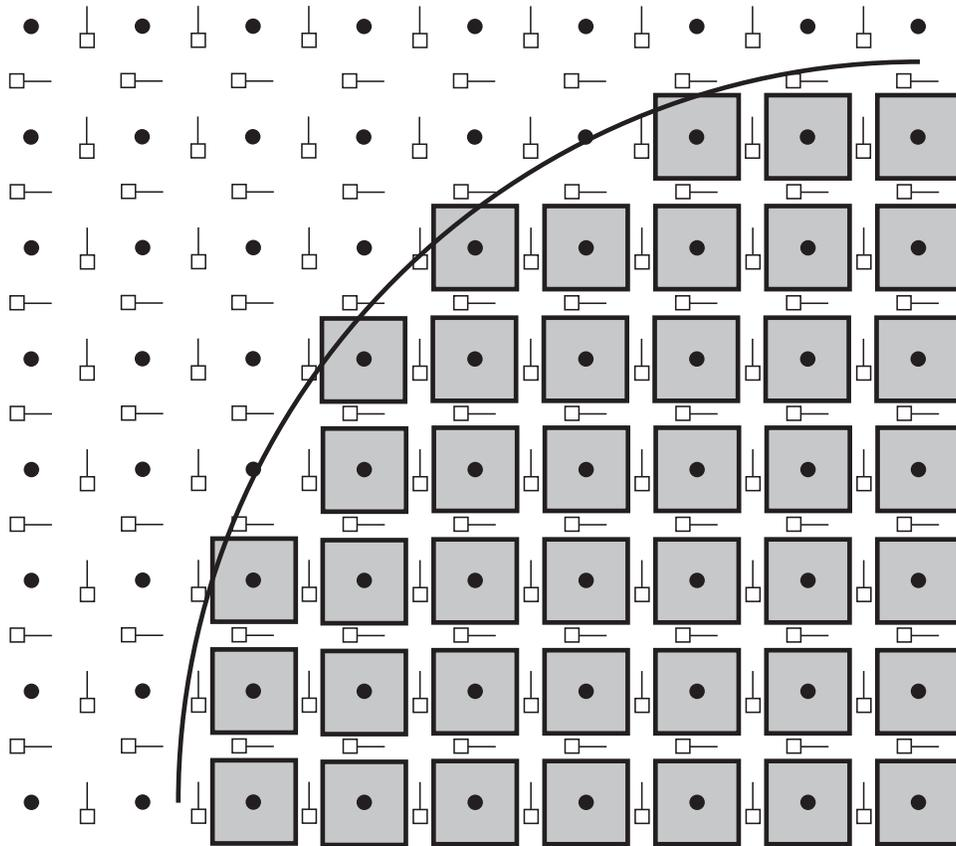
Figure 8.12:  $TM^z$  grid with a PEC object. The PEC is assumed to exist below and to the right of the curved boundary. The PEC is realized by setting to zero the  $E_z$  nodes that fall within the PEC. The nodes that would be set to zero are surrounded by gray boxes.
