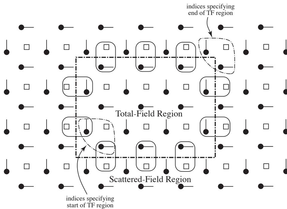
Figure 8.11: TFSF boundary in a  $TE^z$  grid. The rounded boxes indicate the nodes that have a neighboring node on the other side of the boundary and hence have to have their update equations corrected.
