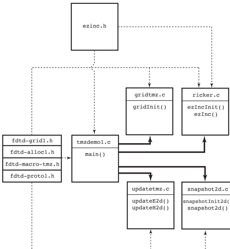
Figure 8.2: The files associated with a simple  $TM^z$  simulation with a hard source at the center of the grid. The four header files with an `fddt-` prefix are lumped into a single box. Not all these files are included in each of the files to which this box is linked. See the code for the specifics related to the inclusion of these files.
