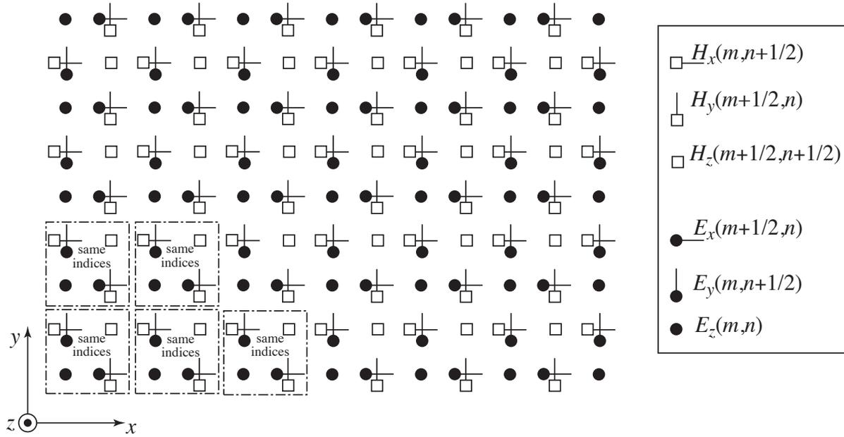
Figure 8.10: Superposition of a  $TM^z$  and  $TE^z$  grid. The symbols used for the nodes is as before. The dashed boxes enclose nodes which have the same indices. Although this is nominally identified as an  $M \times N$  grid, only the  $E_z$  array has  $M \times N$  nodes.
