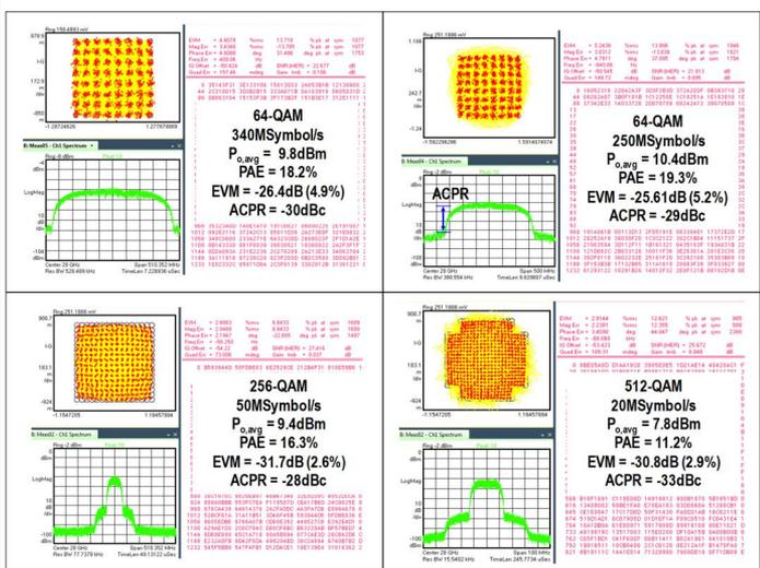
Figure 26.4.5: Measurement results of demodulated signals at 28GHz.
