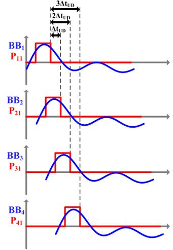
Fig. 4. Offset-sampling technique used to implement TD.
