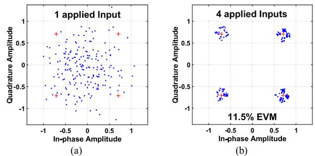
Fig. 15. Measured constellation of a desired 4-Mb/s QPSK signal in the presence of a 12-dB stronger wide modulated BW interference. (a) One applied input (without SpICa). (b) Four applied inputs (with SpICa).
