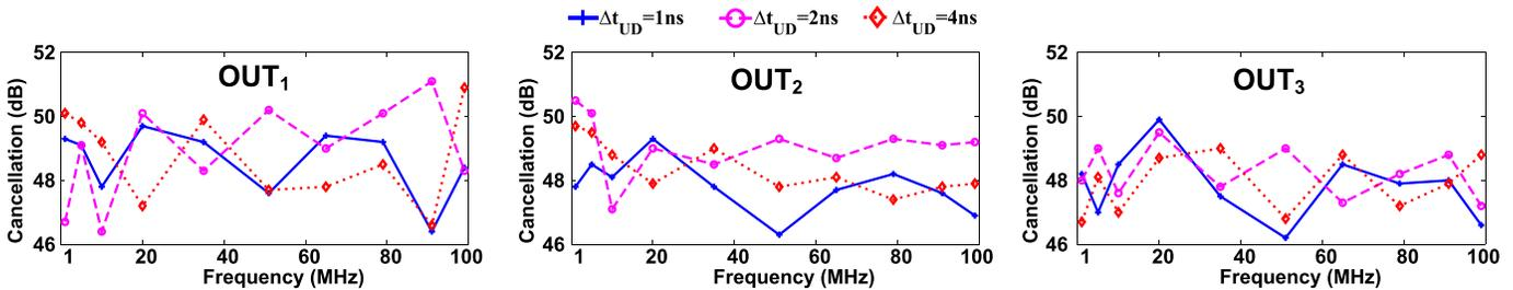
Fig. 13. Measurement results of the single-tone undesired signal SpICa performance versus frequency for three cases of  $\Delta t_{UD}$ .
