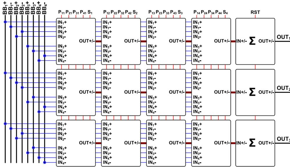
Fig. 5. THM realization through differential analog MAC implementation.
