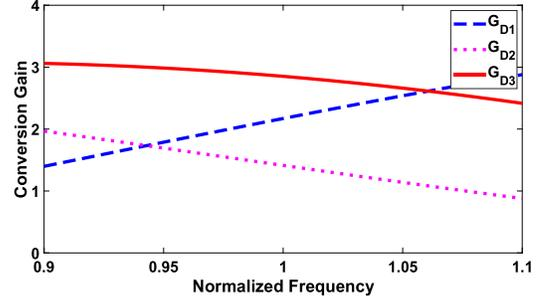
Fig. 17. Desired signal conversion gain versus normalized frequency over 20% fractional BW in the proposed SpICa scheme.
