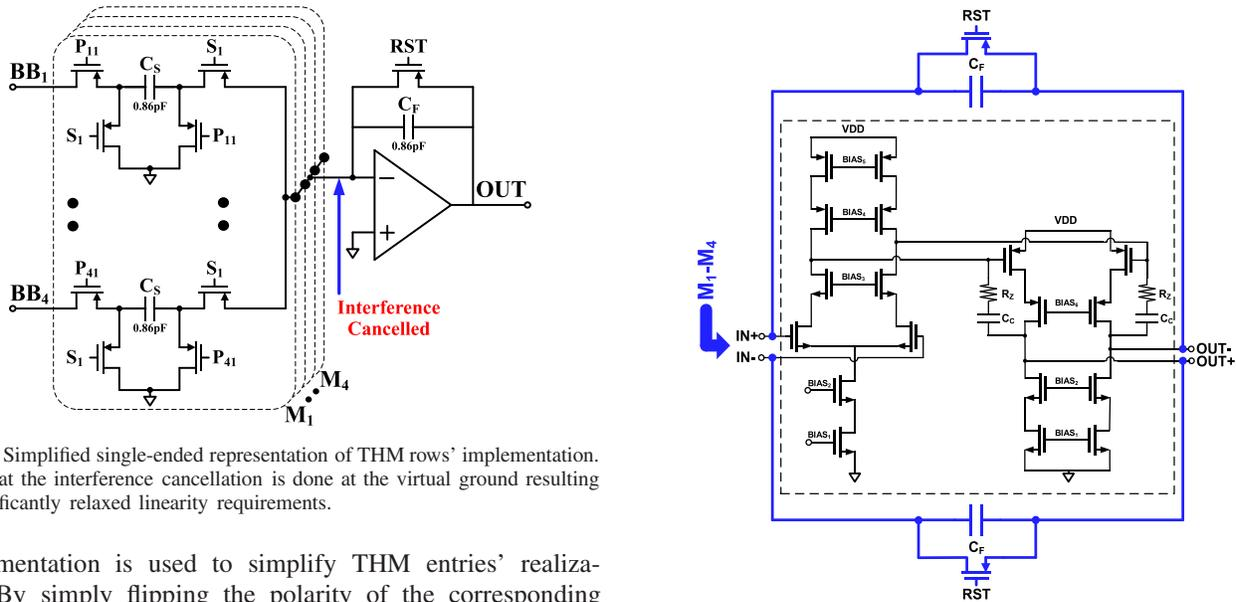
Fig. 6. Simplified single-ended representation of THM rows' implementation. Note that the interference cancellation is done at the virtual ground resulting in significantly relaxed linearity requirements.
