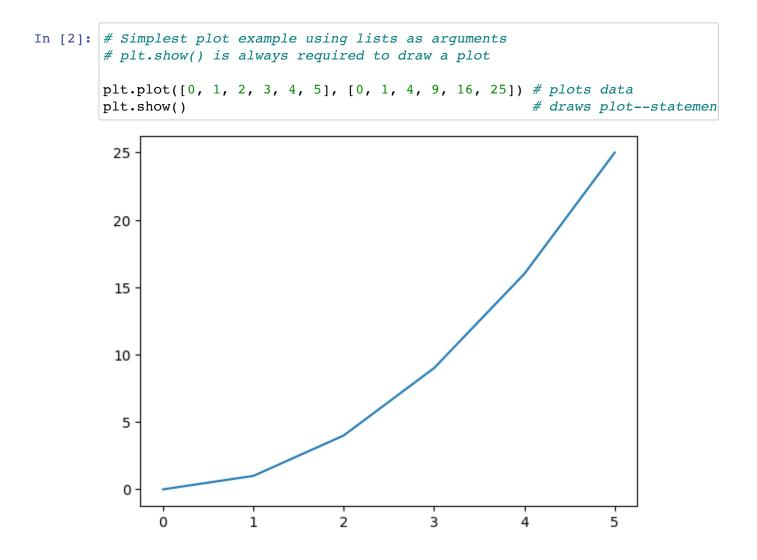
plt.plot() is used to plot the data. Note that plt.show() is always required as the last statement. If you forget to use it, the plot won't be drawn. The list arguments we used above represent the x and y points. Thus, we could have also used the following.
