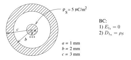
We're asked for the electric flux density in the dielectric right next to the inner conductor, so we use the second boundary condition:
