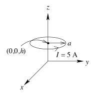
First make a sketch and choose the appropriate coordinate system. Next write down the appropriate form of the BS law. In this case we have a line current so:
