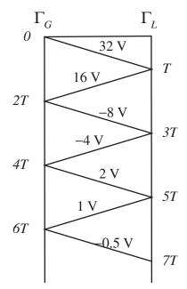
(b) (4 pts) What is  $V_L$ , the line voltage at the load, at t = 0 s?
